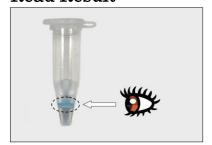
Compare with the top layer of resin (area of dotted circle-line in the left picture) and **Color Index Card**. If necessary, overlap **AgriChem** onto the **Color Index Card**.
