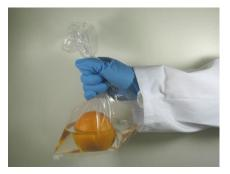
⑤ Pour 100ml of the extraction water in the bag into beaker (of 100mL).
