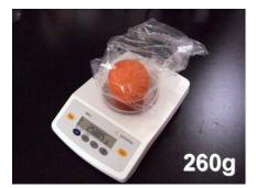
3 Add an equal weight of water \*1(1g=1mL) into the bag by beaker (of 100mL)
