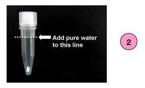
\*\*Prepared **Solution-2** is not possible to preserve nor re-use. Adjust only the inspection numbers of this solution and use once and daily. Do not re-use.
