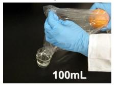
⑥ For removing solid contaminants in extraction water, set the filtration pack onto beaker (of 200mL) and add whole extraction water to the filtration pack. Collect more than 10ml of filtrated extraction water and discard the filtration pack and the remaining extraction water on filter.
