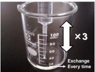
(3) The remained water in the **Column Syringe** needs to be completely drained by moving the piston of the syringe up and down.
