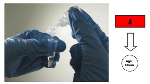
(9) Compare the color of top layer of AgriChem with the Color Index Card
